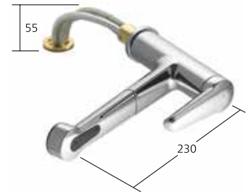
Lever mixer – Detachable for installation below windows – detached 55 mm – Pull-out spray with KWC jetclean – up to 600 mm pull-out length – automatic diverter reset – hose surface to fit faucet surface – Hose guide, swivelling 130°
